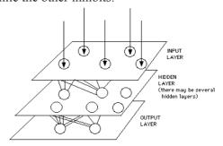
Figure 1:- A Simple Neural Network Diagram. aAll artificial neural networks have a similar structure or topology as shown in Figure 1. In that structure, some of the neurons interface to the real world to receive its inputs. Other neurons provide the real world with the network's outputs. This output might be the particular character that the network thinks that it has scanned or the particular image it thinks is being viewed. All the rest of the neurons are hidden from view.
