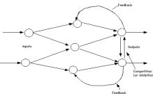
Figure 2:- Simple Network with Feedback and Competition. The way that the neurons are connected to each other has a significant impacton the operation of the network. In the larger, more professional softwaredevelopment packages the user is allowed to add, delete, and control these connections at will. By "tweaking" parameters these connections can be made to either excite or inhibit.
