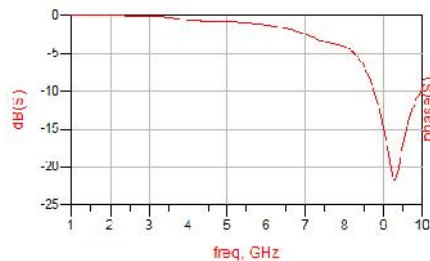
Fig. 9 Return loss S11 antenna simulation
